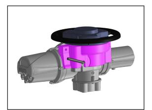
**Step 3** Fit upper handwheel/ declutch lever side Gearcase Cover (FRIQ1T-2100).
