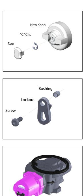
Remove center caps from existing plastic knobs. Remove "C" clips and actuator knobs and retain for re-installation. Remove knob shafts and plastic washers.
