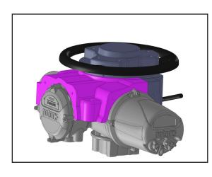
Attach the terminal side of the upper Gearcase Cover (FRIQ1T-2101) next to motor with (2) - M8 x 40 socket head cap screws.
