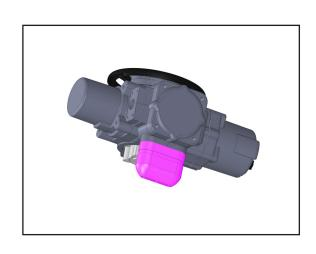
Install the triple conduit cover (KMCP2). Use internal clamps to attach to cables. Place second half and use band clamp to secure. Use 3M Caulk to fill unused holes in cover.
