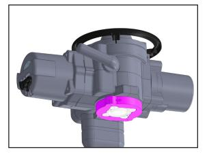
Install Thrust Base Cover (FRIQ2T-2504) using (2) - M6 x 30 socket head cap screws.
