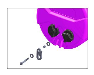
Install lockout plate with original bushing, washers and (1) - M6 x 60 screw to the K-MASS Electronics Cover. Apply blue Loctite thread locker (included) to this bolt only (important).
