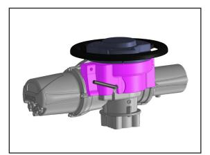
**Step 3** Fit upper handwheel/ declutch lever side Gearcase Cover (FRIQ2T-2100).
