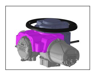
Attach the terminal side of the upper Gearcase Cover (FRIQ2T-2101) next to motor with (2) - M8 x 40 socket head cap screws.
